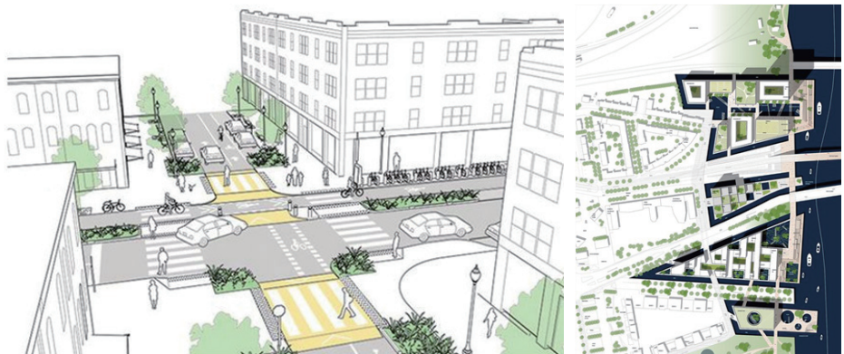
<그림 62> Raised Intersections explained and illustrated in the NACTO Urban Street Design Guide 54)
